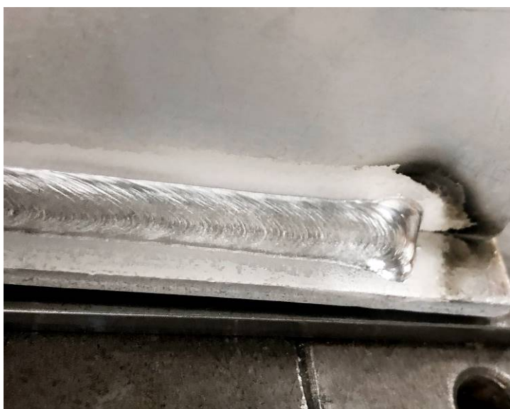
Fig. 2: Aluminum fillet weld with DP-Fast
