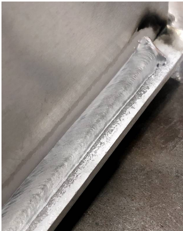
Fig. 1: Aluminum fillet weld with DP-Fast
